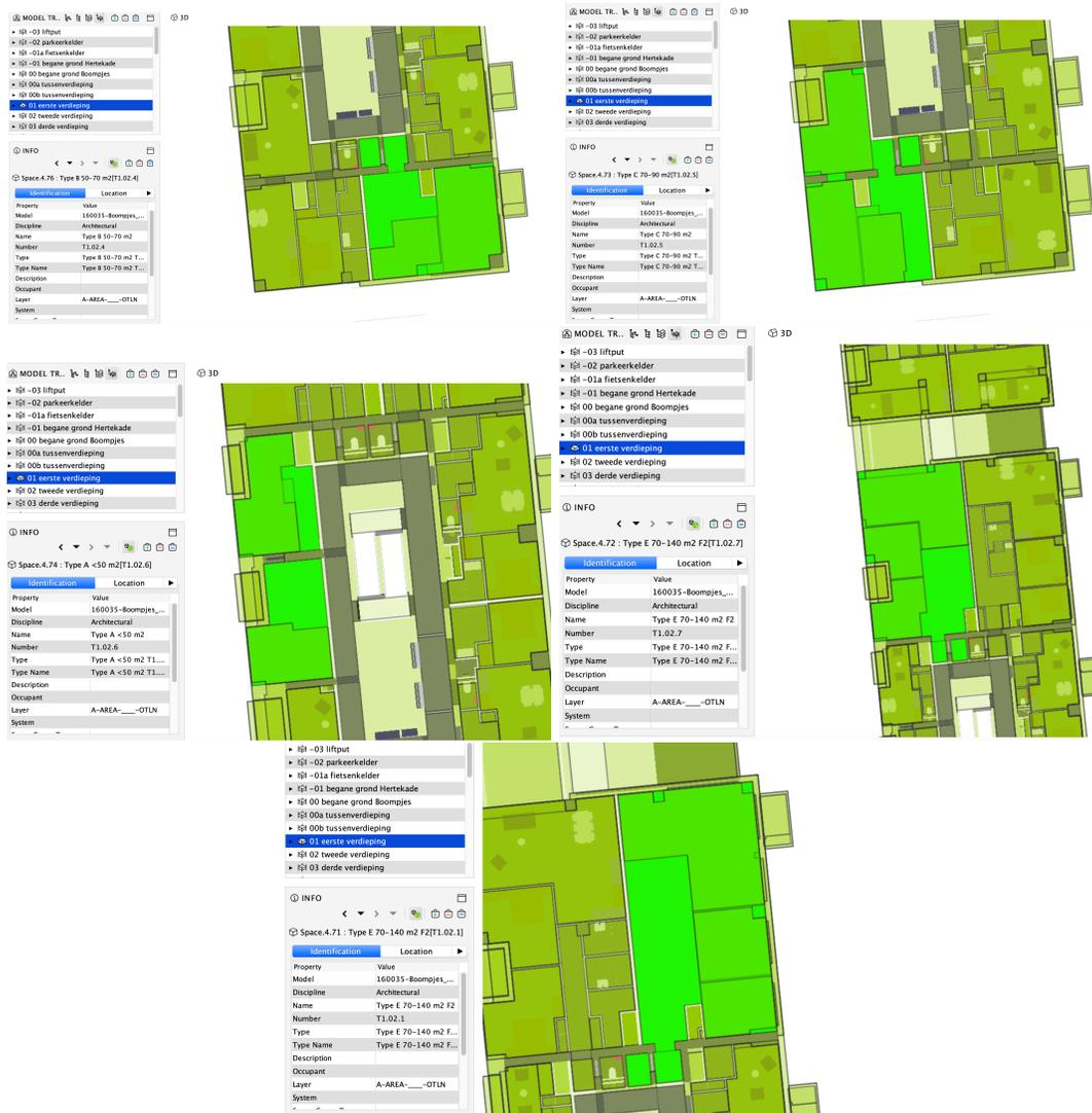
Figure 32: *IfcSpaces* representing apartments. It is possible to notice how the gross floor area is not corresponding to the enclosed volume.
