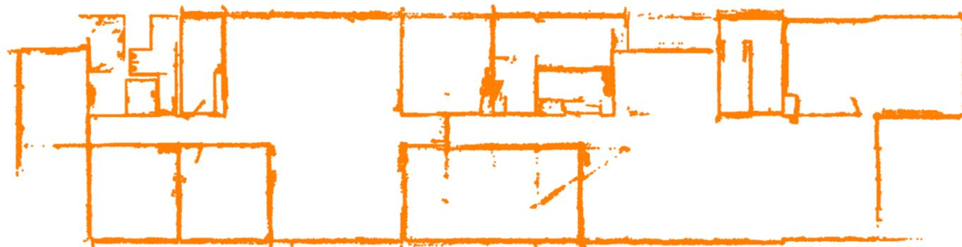
Detected walls from 2nd iteration (top view)
