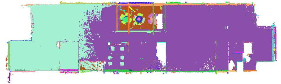
Modified laser points by removing points behind the surfaces
