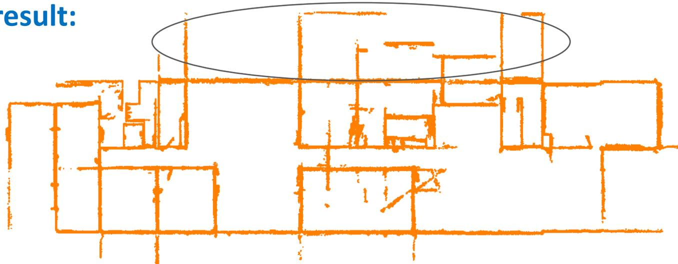
Detected walls from 1st iteration (top view)
