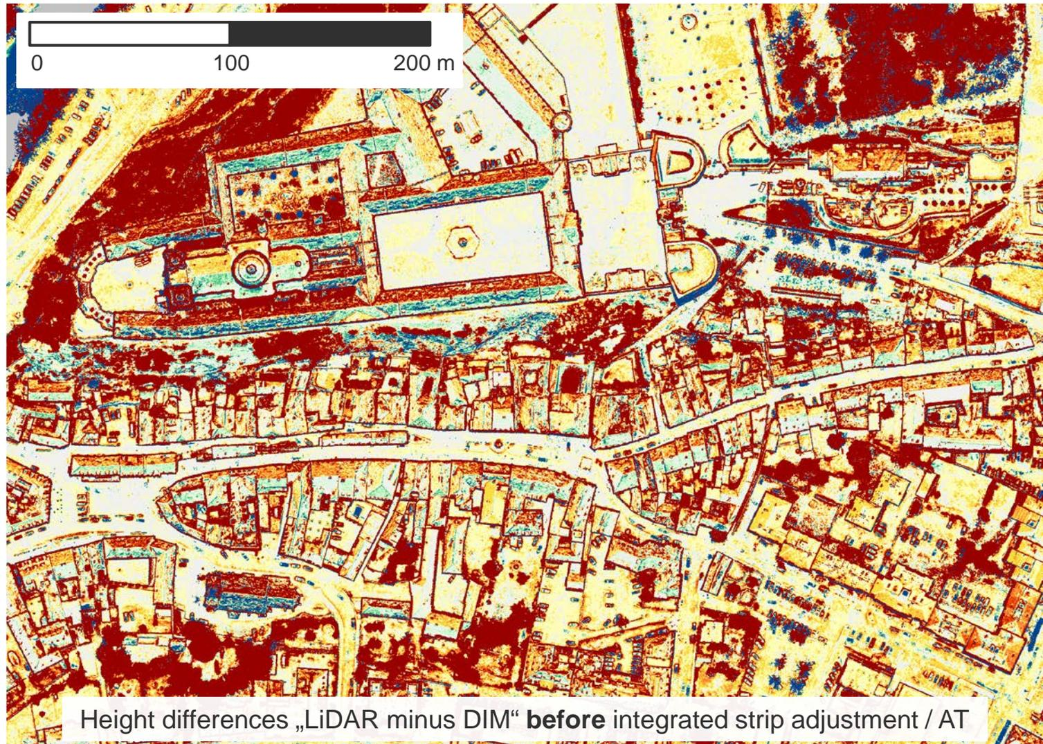
Height differences „LiDAR minus DIM“ **before** integrated strip adjustment / AT
