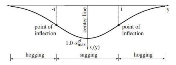
The transversal ground settlement trough profile (adapted by Attewell et al. (1986) and Mair et al. (1996)).
