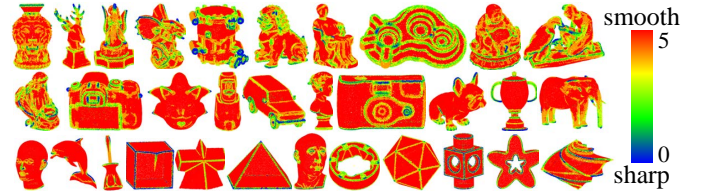
Fig. 5: The geometric feature levels (0-5) of each point in the training dataset. The lower geometric feature levels (in blue) represent sharper regions.
