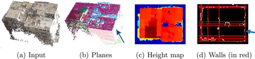
**Fig. 4.** Detection of missing walls. The arrow indicates a missing wall.
