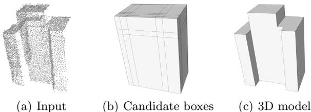
**Fig. 8.** Reconstruction of a single building from airborne LiDAR data.
