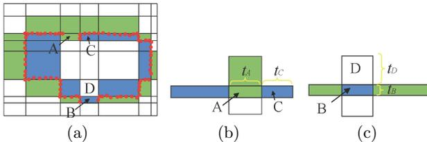
**Fig. 6.** A 2D illustration of holes and protrusions. Box A is misclassified as *negative* resulting in a hole; box B is misclassified as *positive* resulting in a protrusion. The thickness values  $t_A$  and  $t_C$  are used to compute the compactness for box pair A-C, and  $t_B$  and  $t_D$  for box pair B-D. Colors indicate different box types, i.e., blue for positive boxes, green for negative boxes, and white for blank boxes.
