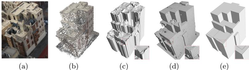
**Fig. 12.** Comparisons with two state-of-the-art methods. (a) An aerial photograph of the building. (b) MVS point cloud. (c) Reconstruction result using the 2.5D dual contouring method [33]. (d) The result from  $L_1$ -based polycube method [9]. (e) Ours.
