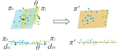
**Fig. 2.** The merging of two planar segments. Two planes  $\pi_0$  and  $\pi_1$  are merged if the angle between them is smaller than a threshold (i.e.,  $\theta < \theta_t$ ), and the distance from their mass centers is less than another threshold (i.e.,  $d_{01} < d_t$  and  $d_{10} < d_t$ ). Then a new plane  $\pi'$  is proposed using a least-squares fitting of the union of the points.
