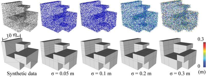
**Fig. 10.** Reconstruction results from a synthetic data with increasing noise levels.
