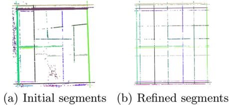
**Fig. 3.** The refinement of the initially extracted planar segments (top-view).
