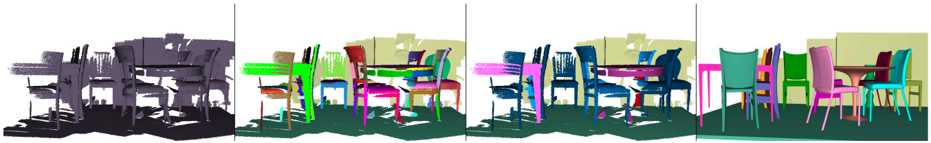
Figure 2: A zoom into the cluttered region of Figure 1 (left), reveal that accurate segmentation and classification are challenging, even for human perception. We initially over segment the scene (mid-left) and search-classify meaningful objects in the scene (mid-right), that are reconstructed by templates (right) overcoming the high clutter.
