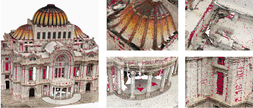
Figure 4.28 – Gap filling visual results for the PB dataset using a 15-point line SE in the x-direction. Red indicates inserted points
