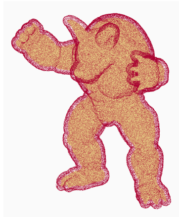
Figure 3.11 – Approximation of the surface-based dilation obtained by subtracting two dilations using spherical SEs one threshold distance apart in radius.
