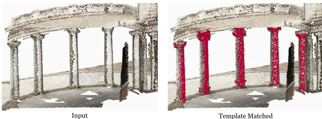
Figure 4.30 – Template matching applied to the PB dataset. Left: input with missing column data. Right: reconstructed points added by template matching shown in red.
