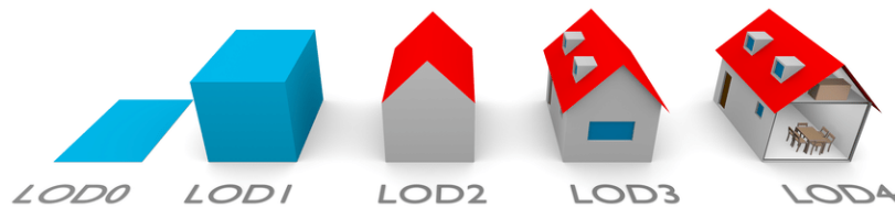
Figure 3.2.: The five LoDs of CityGML 2.0, adapted from (Biljecki et al., 2016)
