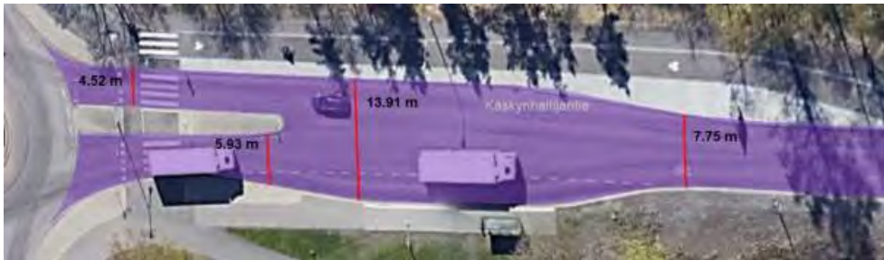
Figure 1.3: Changes of road width, figure from Chatzidiakos [2021].
