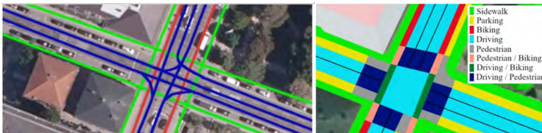
Figure 2.5: Linear semantic enrichment (left) and areal semantic enrichment (right) of TrafficSpace coloured by function attributes in CityGML. Figures from Beil et al. [2020].
