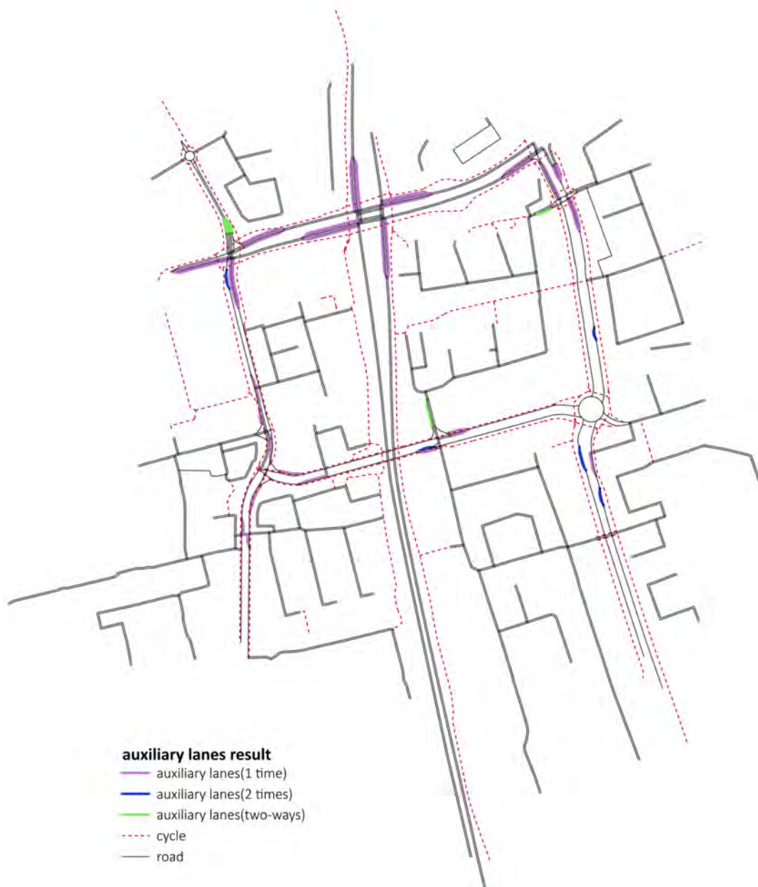
Figure 6.16: Results of lane modification for the auxiliary lanes to align with 'through' lanes.
