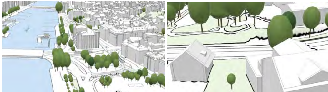
Figure 1.5: Model details of 3D City model of Zurich, the blurred road boundary indicates the poor quality of the road model.
