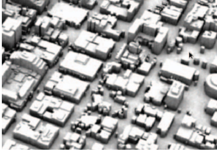
Figure 2.19.: Generated building envelopes using clustering algorithms (Poullis 2013)
