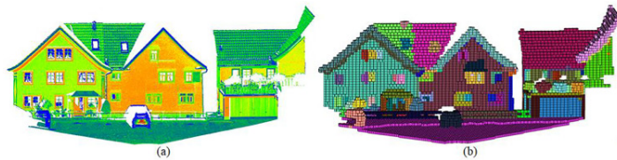
Figure 2.13.: Results of point cloud-based voxelisation(Wang et al. 2015)
