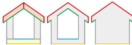
Figure 2.8.: Extracting building envelope by using space partitioning (Donkers et al. 2015)
