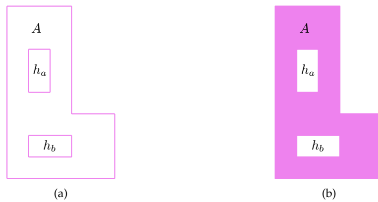
Figure 3.27: An example of using polygonizer to polygonize a set of line segments. (a) A set of line segments. (b) The resulting polygon of Polygonizer containing two interior holes.
