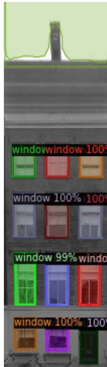
Figure 1.2.: Façade parsing example: identification and segmentation of windows and doors. The aim in this thesis is to count the number of storeys from the repetitive occurrence of windows and doors.
