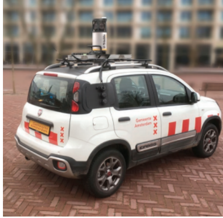
Figure 5.1.: The car of the City of Amsterdam that is used to capture SVI from Amsterdam, equipped with a 360° Trible MX7 mobile imaging system. Source: [ Geospatial, 2022 ]
