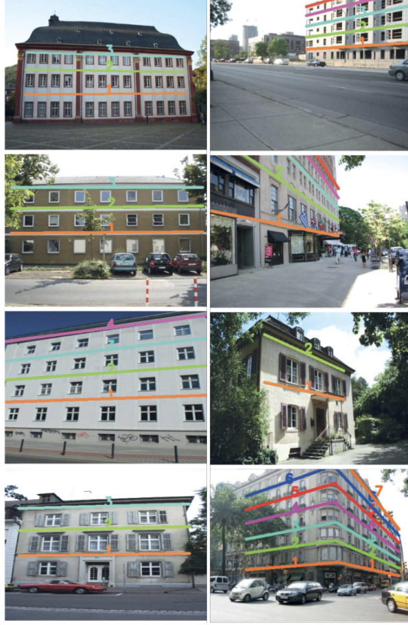
Figure 3.6.: The results of floor-level line detection with FloorLevel-Net, on more orthogonal view images (left) and perspective view images (right). Note how the floor-level line number corresponds to the number or count of the storey it is assigned to. In most cases, the highest floor-level line number corresponds to the floor count. Adapted from [Wu et al., 2021].
