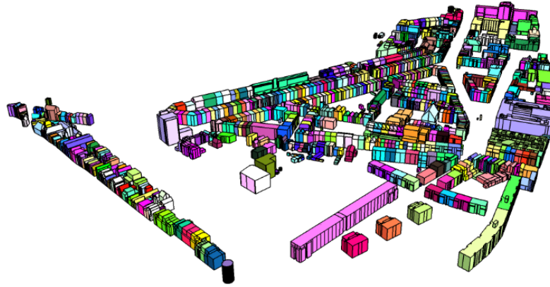
Figure 2.7: A LCC viewer to evaluate the topologically reconstructed CityJSON files [Vitalis et al., 2019]
