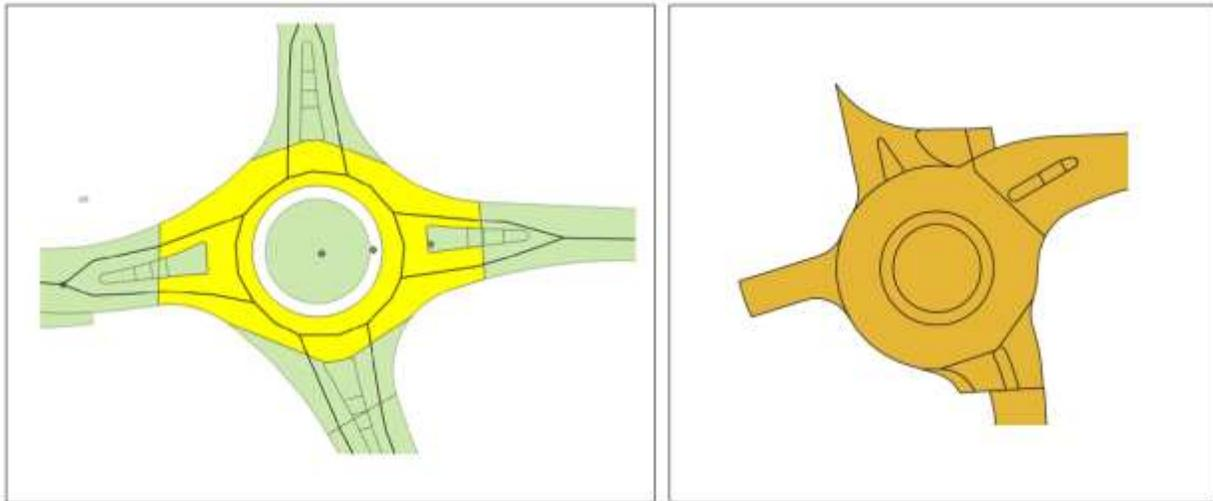
*Figure 29 Roundabout polygons can have a rather complex structure. In many datasets more than 3-4 polygons are used to represent them. This will cause problems to our standardization methodology. We need to identify roundabouts and then create a new, simple roundabout polygon.*
