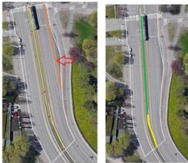
Figure 22 Road where change in number of lanes exists. Original road centerline (left), my view on how this centerline should be divided into 2 centerlines (right). Source: Google earth V 6.2.2.6613
