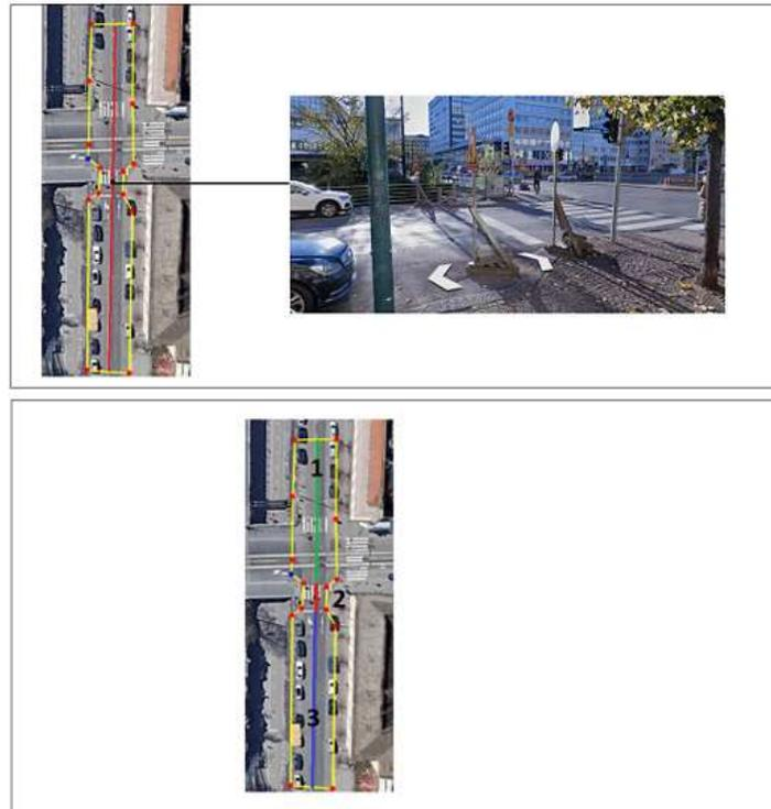
Figure 23 Case where a narrow spot exist in a road network. Original centerline (top left), ground truth of how the original centerline should be divided into 3 new clusters (bottom). Source: Google earth V 6.2.2.6613
