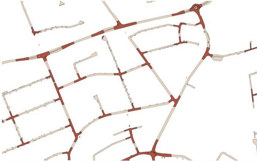
*Figure 33 New intersection polygons created after computing the intersection between intersection node buffers and dissolved initial areal geometries*
