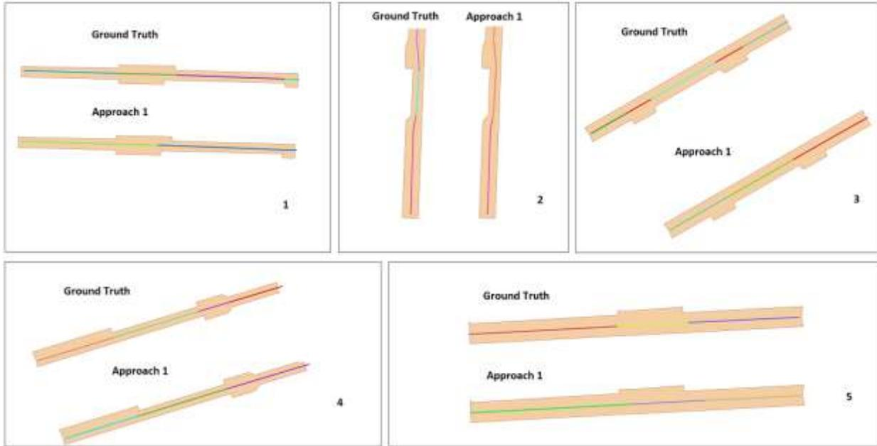
Figure 95 Results of clustering approach 2 for polygons of category B. The final index is 0.72. In most of the cases a different strategy is followed by this approach. In most of the cases the approach 2 resulting clusters seem quite different and the parking spot is not identified as a different cluster (case 1,2,3,4). Only one out of 5 cases seem to have identical results.
