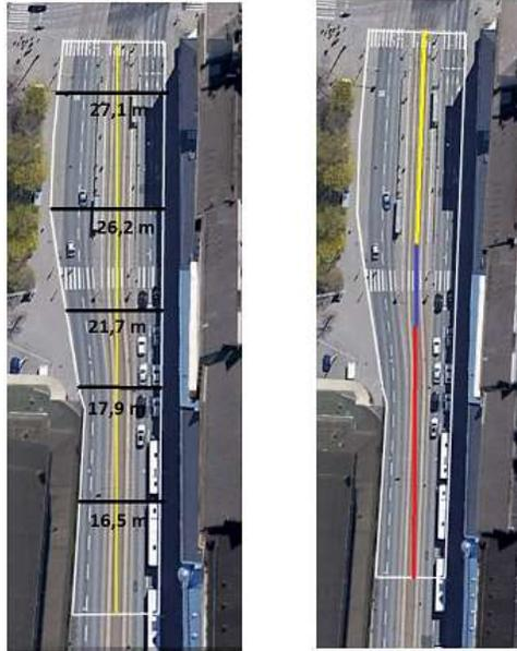
Figure 20 My view on how original road centerline (left) should be subdivided into 3 clusters based on the notable width changes that occur on that road (right). Source: Google earth V 6.2.2.6613
