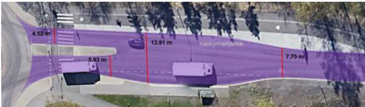
Figure 1: Road called Käsäynhaltijantie located in Helsinki (Finland). Different width measurements are available for that road. The width interpretation of this road depends on the road user (application that needs width information).
