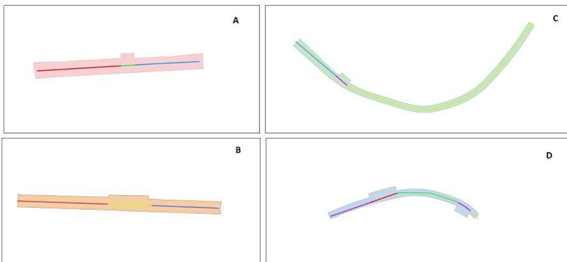
Figure 92 Road polygons of this case are divided into 4 categories. Straight roads with maximum of 2 on-street parking spots (A), Straight roads with more than 2 on-street parking spots (B), Curved roads with maximum of 2 on-street parking spots (C), Curved roads with more than 2 on-street parking spots (D).
