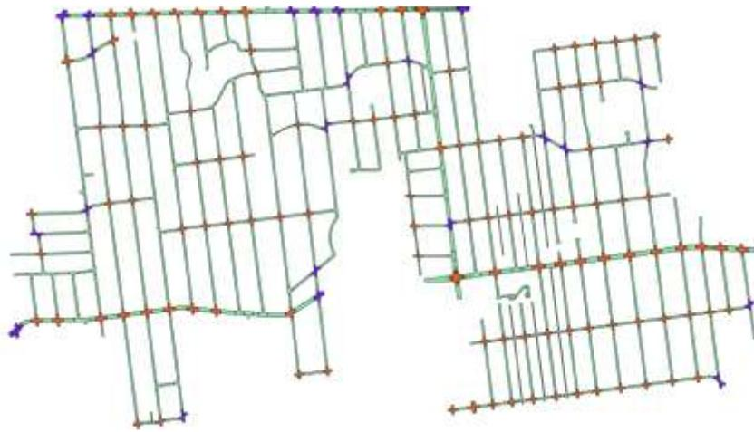
Figure 81 Sample area contain the intersection polygons that identification approach was tested with. Cross intersection polygons in orange color and X intersection polygons in blue color.
