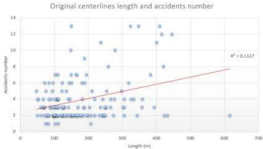
Figure 100 Graph shows the relation between length of a road centerline and the number of accidents that occur. We can claim that while e the road length increases, the number of accidents increases as well.
