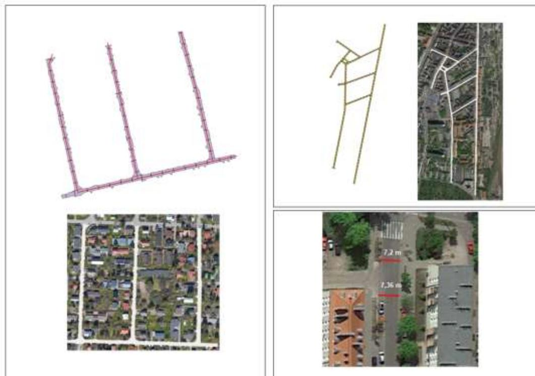
Figure 63: 100 measuring lines was defined as ground truth in order to compared with measuring lines result from initial methodology (top right). 48 measuring lines correspond to roads located in Helsinki (Left), 52 measuring lines correspond to roads located in Poznan (right)
