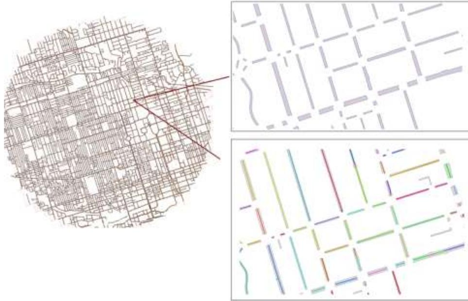
Figure 112 Road centerlines clustered based on width, intersection polygons excluded
