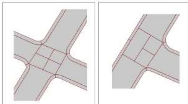
*Figure 73 A cross intersection is modelled with 4 different polygons while T intersection is modelled with 3 different polygons in the dataset of Montreal*
