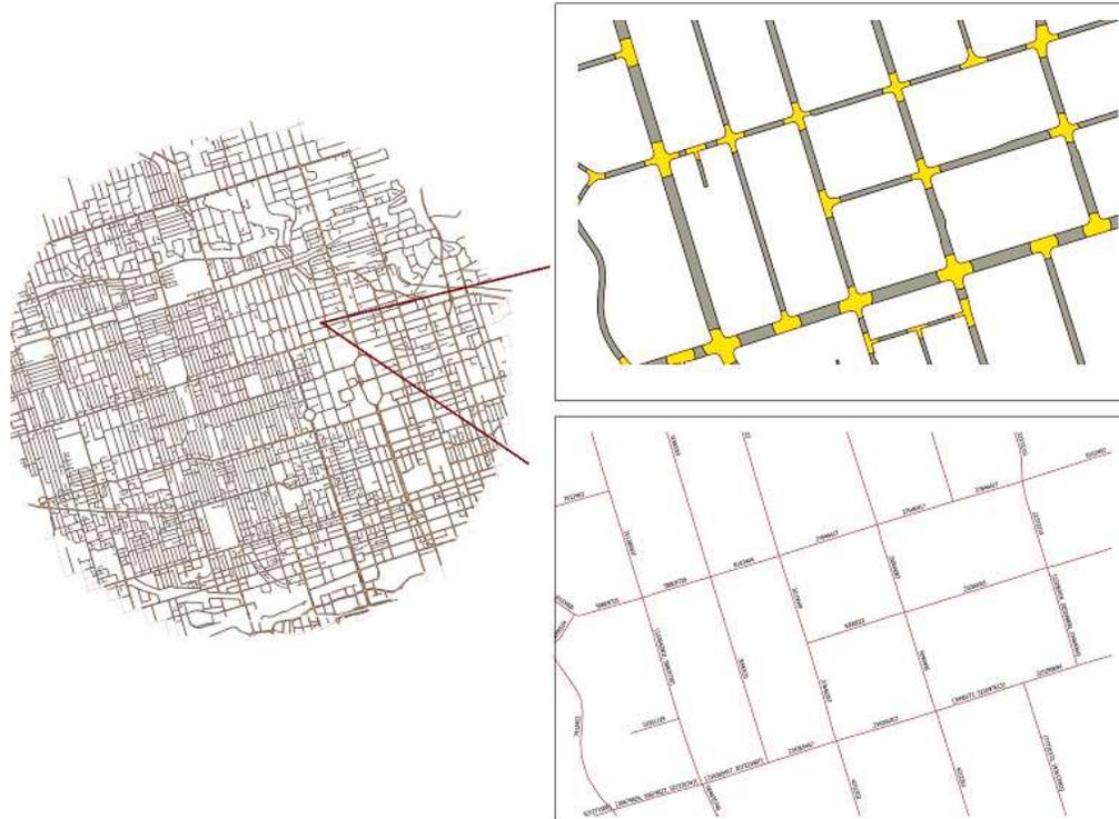
Figure 102 For dataset 1 width is estimated for the original road centerlines (extend from one intersection to another) using the original road polygons
