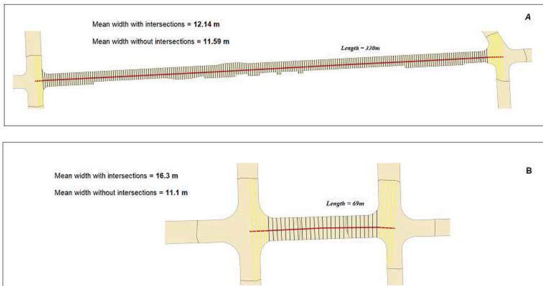
Figure 117 The mean width estimation for a long road (A) is changing only by 0,5 meters after removal of intersection polygons. For a shorter road (B) of length less than 70 meters, the final width estimation differs more than 5 meters
