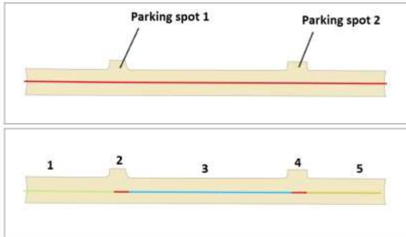
Figure 91 Road polygon that contains 2 parking spots and the initial modelling of one single centerline (Top). Our ground truth that defines a new road cluster every time that a parking spot is present (Bottom). In order to make sure whether there is a parking spot we used satellite images from Google earth (<https://earth.google.com/web>)
