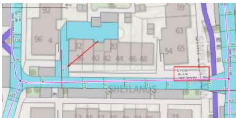
Figure 19 Methodology of ten lines road width calculations with vector data Source: Hoffmans W. [25]
