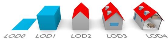
Figure 1: A building represented in LOD<sub>0</sub> to LOD<sub>4</sub> (image from Biljecki et al. [2016b]).
