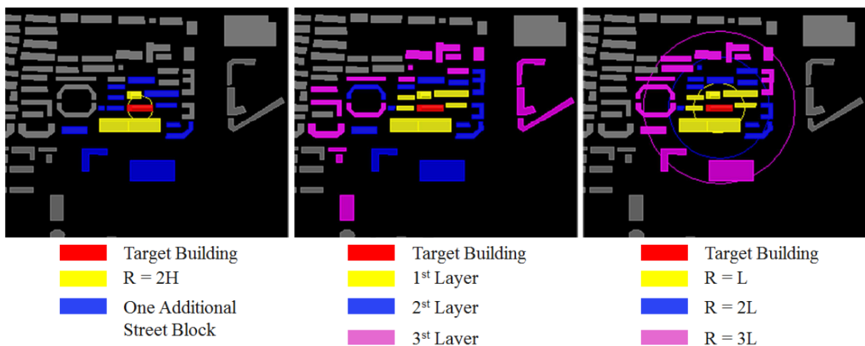
Figure 2.13: The definition of the influence zone by Tominaga et al. (2008) (left), Tong et al. (2016) (middle) and Liu et al. (2018) (right), from Liu et al. (2018).
