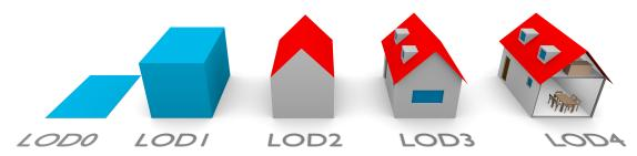
Figure 1: The five LODs of CityGML 2.0. The geometric detail and the semantic complexity increase, ending with the LOD4 containing indoor features.
