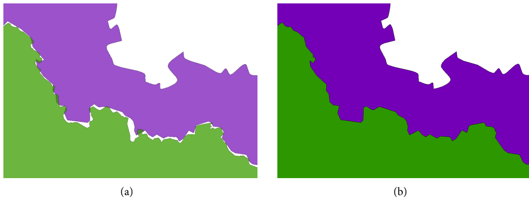
Figure 13: (a) The same dataset as Figure 10(a). (b) Edge-matching performed with a repair operation where the label assigned to a problematic region is the one of the adjacent neighbour having the longest common boundary. Notice the differences with Figure 10(d).
