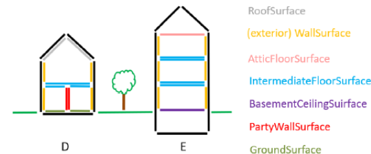
Figure 21. Schematic examples of surfaces modelled using different classes.
