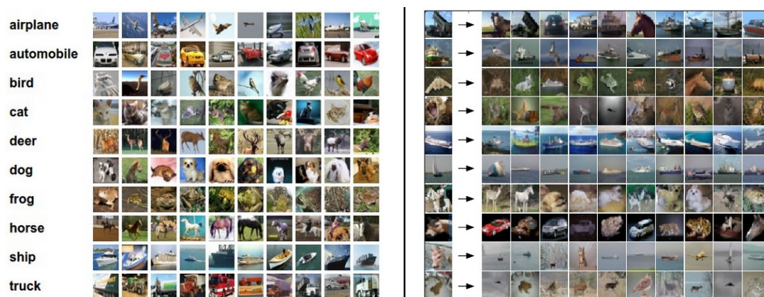
Figure 4: Left: Example images from the CIFAR-10 dataset. Right: first column shows a few test images and next to each we show the top 10 nearest neighbors in the training set according to pixel-wise difference.
