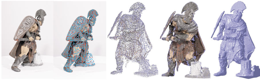
Figure 1. Overall approach. From left to right: a sample input image; detected features; reconstructed patches after the initial matching; final patches after expansion and filtering; polygonal surface extracted from reconstructed patches.
