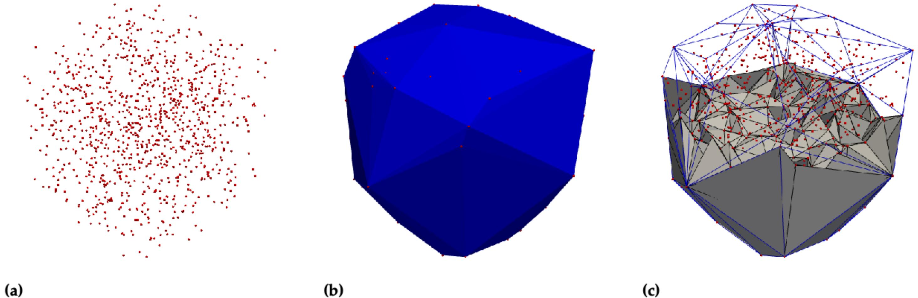
**Figure 3.8:** (a) A set of 1000 points randomly distributed in a cube. (b) Its convex hull. (c) The Delaunay tetrahedralisation of the points, 'sliced' in the middle and the upper tetrahedra removed (to be able to visualise the interior).
