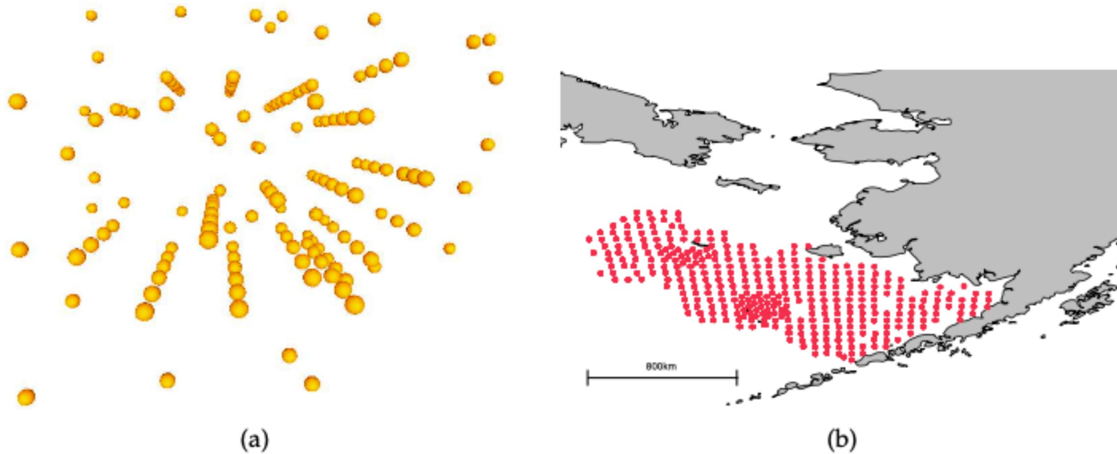
Figure 10: **(a)** Example of a dataset in geology, where samples were collected by drilling a hole in the ground. Each sample has a location in 3D space ( $x - y - z$  coordinates) and one or more attributes attached to it. **(b)** An oceanographic dataset in the Bering Sea in which samples are distributed along water columns. Each red point represents a (vertical) water column, where samples are collected every 2m, but water columns are about 35km from each other.
