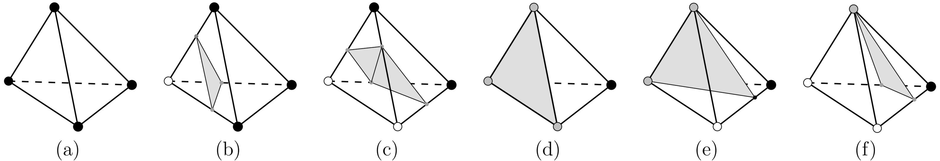
**Figure 3.15:** Potential isosurface (for an attribute value  $v$ ) extracted for one tetrahedron. Black vertex means that the attribute of this vertex is below  $v$ ; white vertex means it is above; and grey that it is equal.
