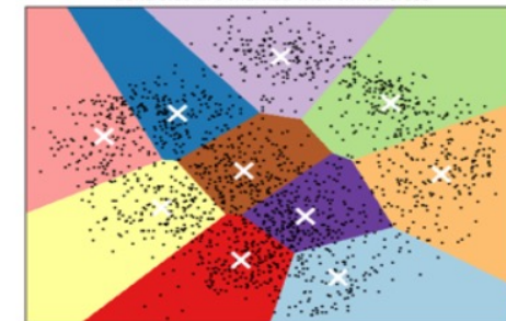
K-means clustering on the digits dataset (PCA-reduced data) Centroids are marked with white cross
