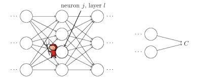
The demon sits at the j-th neuron in layer l. As the input to the neuron comes in, the demon messes with the neuron's operation. It adds a little change  $\Delta z_j^l$  to the neuron's weighted input, so that instead of outputting  $\sigma(z_j^l)$ , the neuron instead outputs  $\sigma(z_j^l + \Delta z_j^l)$ . This change propagates through later layers in the network, finally causing the overall cost to change by an amount  $\frac{\partial C}{\partial z_j^l} \Delta z_j^l$ .
