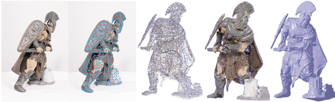
Figure 2.7: PMVS - overall approach. From left to right: a sample input image; detected features; reconstructed patches after the initial matching; final patches after expansion and filtering; polygonal surface extracted from reconstructed patches.[2]
