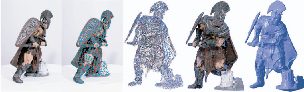
Fig. 1. Overall approach. From left to right: A sample input image, detected features, reconstructed patches after the initial matching, final patches after expansion and filtering, and the mesh model.
