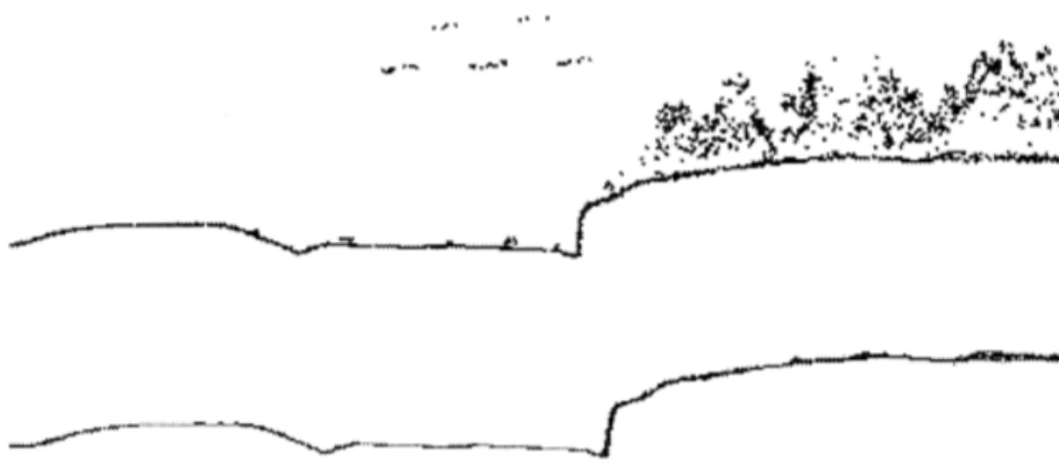
Figure 1: Cross-section of a terrain with lamp posts and trees before (top) and after (bottom) ground filtering (Axelsson, 2000).
