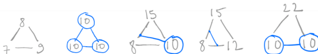
Figure 4: Different cases when extracting an isoline at elevation 10m for a TIN. The grey values are the elevation of the vertices forming one triangle, and the blue lines and vertices are the ones extracted for that triangle.
