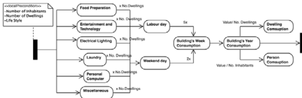
Figure 6.14.: Extract of the activity diagram for estimation of energy consumption source: Own graph
