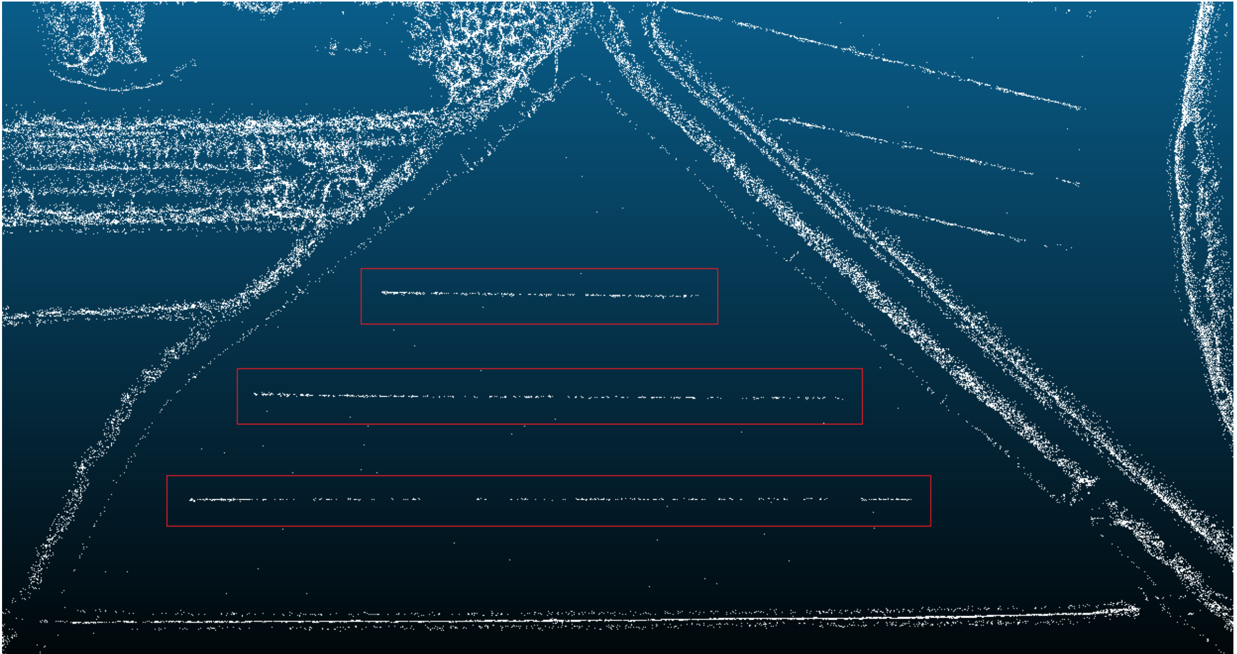
Figure 12: Dry channels identified by MAT (in red rectangles). Channels are fragmented.
